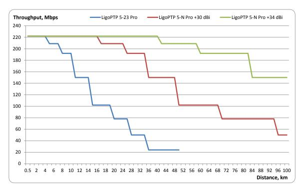
The graph above represents LigoPTP 5-23 PRO and LigoPTP 5-N PRO capacity at different distances. The calculations were done with a 15 dB fade margin and no interference on the link.
